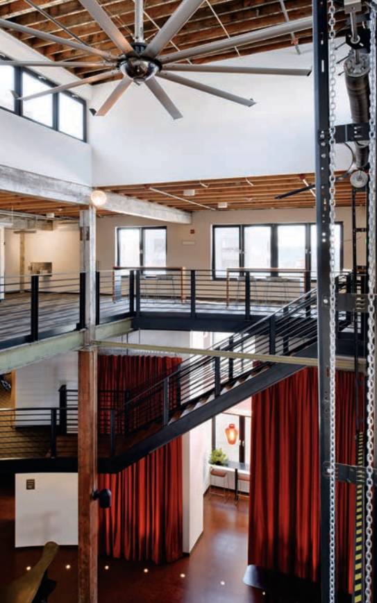
The 18 ft x 25 ft central forum opening on the third floor allows for airflow and daylighting to the lower levels.
