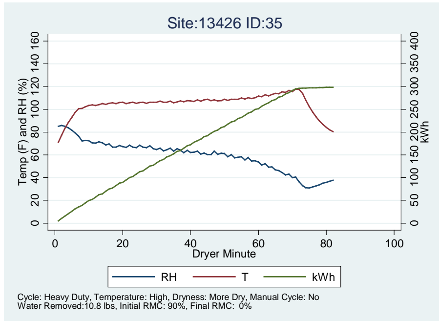
Figure 60. Dryer Single Cycle Energy Profile – Multi-Run Cycle
